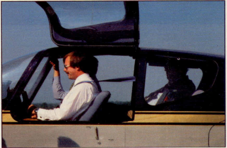
The front seats are by far the most comfortable; rear-seat passengers face a tight squeeze in this prototype Tobago. U.S. versions of the final design will have vertically adjustable seats.
