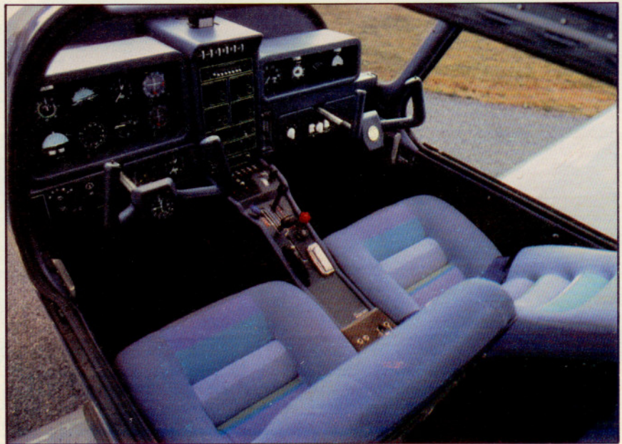
Gull-wing doors, reclining seats and sports-car-style power console mark the interior. The panel, divided into three hinged modules, is designed for easy maintenance of the instruments.
